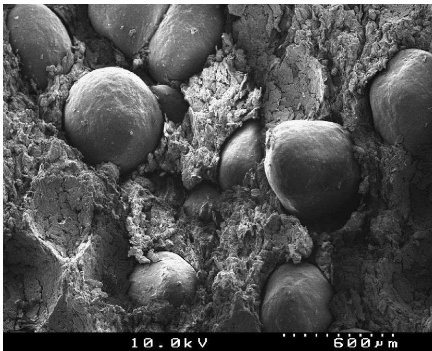
Fig. 7. SEM photographs of the broken tablets containing propranolol HCl pellets, coated with Kollicoat ® SR 30 D (10% w/w triethyl citrate, coating level 20% w/w, tableting excipient Avicel PH 200, pellet content 50%, compression force 15 kN).
